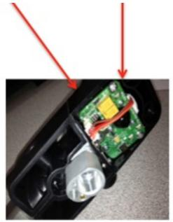
New stronger nozzle/barrel design eliminates the need for a peek insert, making the new barrel easy to identify.
